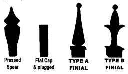
Finials are made of a heavy, aluminum metal and powder coated.
