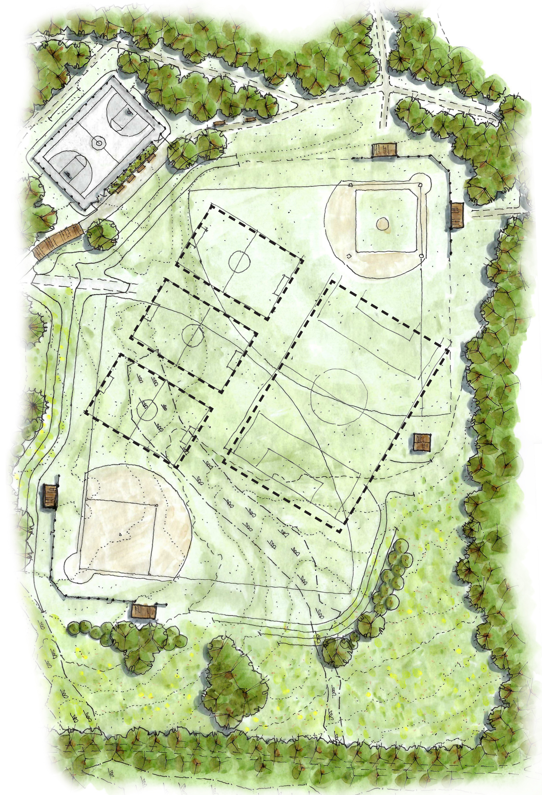
Multi Use Athletic Fields Layout B Softball & Baseball with (1) U10 & (3) U6-8 Fields (Scale: 1"=40')
