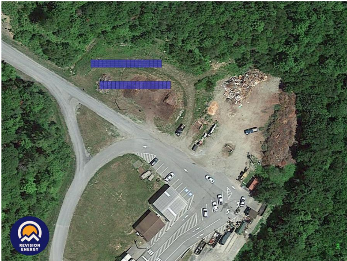
Figure 1: Engineer's rendering of proposed 53.28 kW Solar Array on the Readfield Transfer Station.
