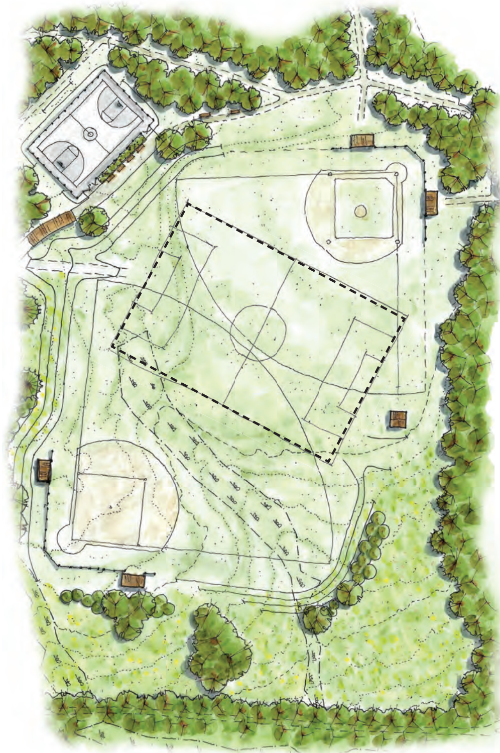
Multi Use Athletic Fields Layout A Softball & Baseball with U12 Field (Scale: 1"=40')
